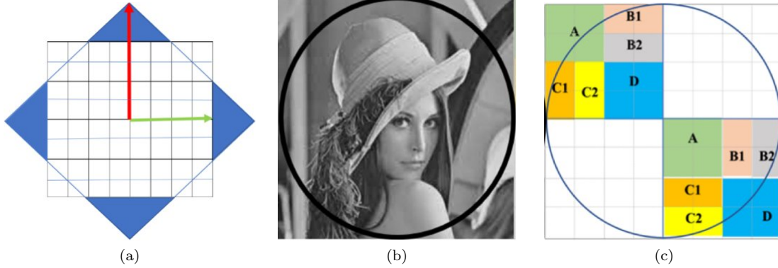
Figure 6: New scheme for embedding vulnerable data from corners of the image, to inside the safe circle of the image.
